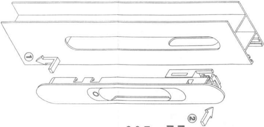
**MISE EN PLACE DE L'ANTI-FAUSSE MANŒUVRE**
